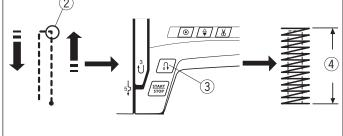
Tacking is used to reinforce pockets, crotches and belt carriers where extra strength is needed.
