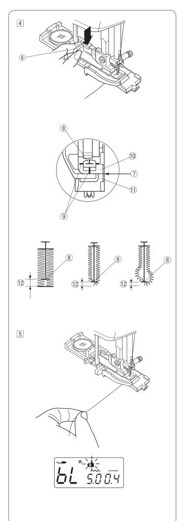
4 Lower the presser foot and pull the buttonhole lever down as far as it will go.
