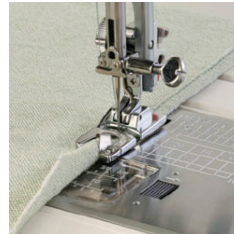
202-081-203 Rolled hem foot with 4 mm width (D2)
