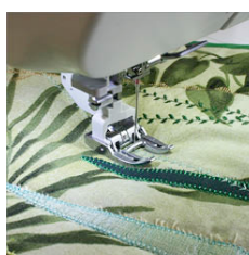
202-236-009 Dual Feed open-toe foot – wide system (UD)
