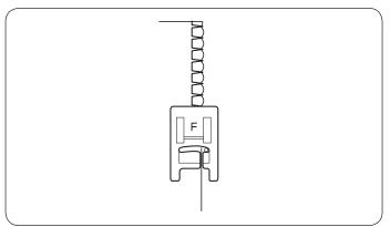
Sew a fine seam in lingerie and lightweight knits. The small seam size stretches and is comfortable to wear.
