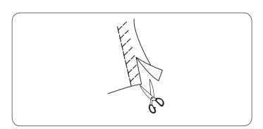
Place your fabric to allow a 5/8" (1.5 cm) seam. Trim excess close to the stitching. Be careful not to cut the stitches.
