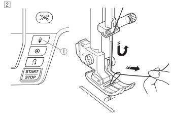
Press the needle up/down button ① twice to lower and raise the needle to pick up the bobbin thread.① Needle up/down button
