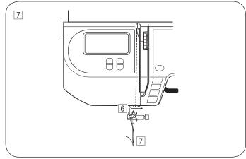
7 Thread the needle from front to back, or use the needle threader (see page 22).
