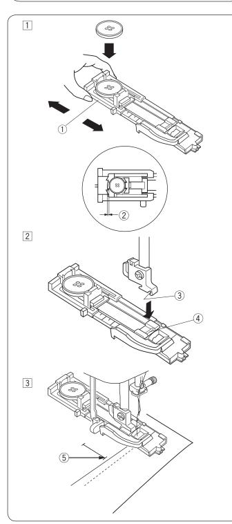
The size of a buttonhole is automatically set by placing a button in the rear of automatic buttonhole foot R.
