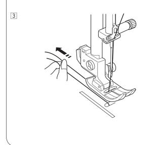
3 Pull both threads 10 to 15 cm (4" to 6") under and behind the presser foot.
