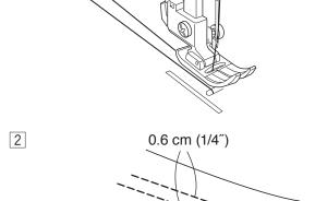
2 Sew two rows of straight stitches 0.6 cm (1/4") apart. Knot the threads at the beginning.
