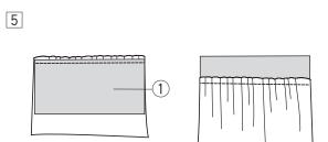
5 Prepare the fabric to attach the gathering. Tighten the thread tension to "4" and decrease the stitch length to "2.4" (default settings). Place the wrong side of the fabric ① under the gathering. Sew the straight stitch between the two gathering Remove the two rows of straight stitches.
