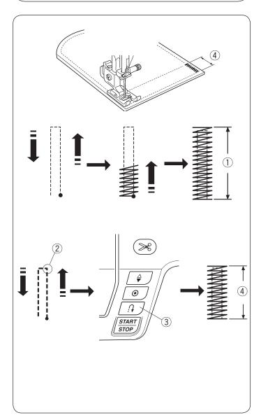
Tacking is used to reinforce pockets, crotches and belt carriers where extra strength is needed.
