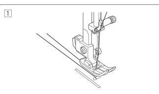
1 Loosen the thread tension to "1" and increase the stitch length to 5.0.
