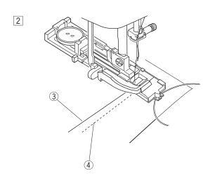
2 Start the machine and sew the buttonhole. Each side of the buttonhole and the bartacks will be
