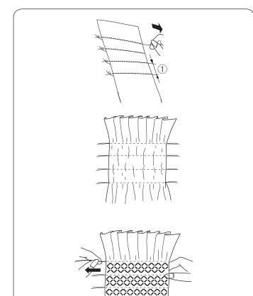
2 Sew down the left side, guiding the fabric so the right hand stitches fall in open space. After finishing the left side, press the mirror image key. Sew down the other side (refer to page 77 for mirror image sewing).
