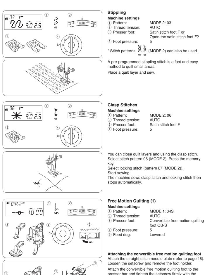
presser bar and tighten the setscrew firmly with the screwdriver.
